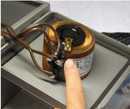
Figure #2 – Live wire resulting in possible contact voltage
